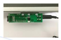
3. Plug the small black plug attached to the SKY Kit into the top socket on the circuitboard at the bottom of the TV.
