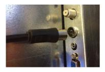
I. Connect one end of the connector cable to the Aerial input of your TV.
