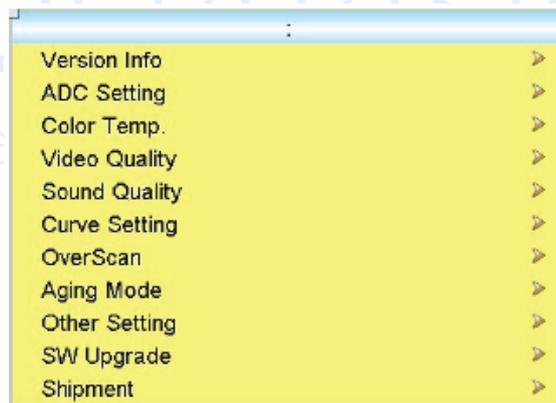
Move cursor to SW Upgrade and press RIGHT key to enter upgrading, please keep power on in the upgrading process, it will take about 1-2 min. When the indicator ligh stops flickering, it means the upgrading is successful, the system will be in stand-by condition, now you need to remove the U disk first, then have AC dump and power on again (this point is very import, or, it will have fake burning)
