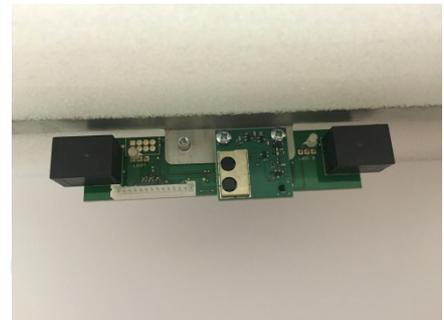
3. When installing this board, dependent on the model and age of the television, you may need to use the spacers and longer screws (supplied). The small board should be installed on the front of the fixings, and the larger board on the rear. Spacers could be used to lift the small board as high up as possible without it being above the front of the screen.
